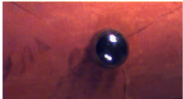
*Figure C. Steel Projectile at Moment of Impact with Concrete Tile.*
