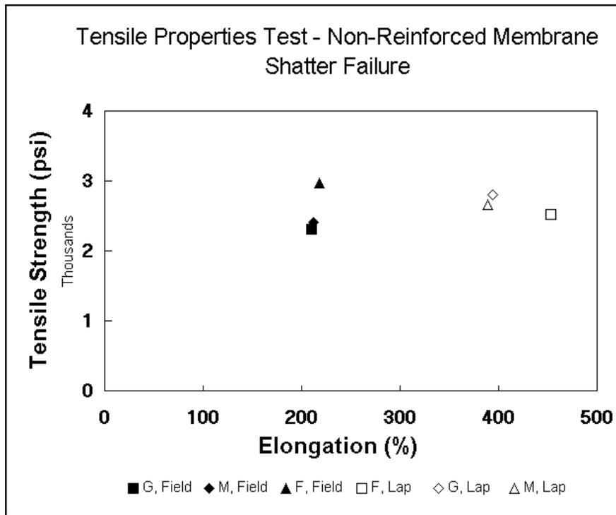
Figure 4, Tensile/Elongation Rates for Non-Reinforced Shattered Membranes.
